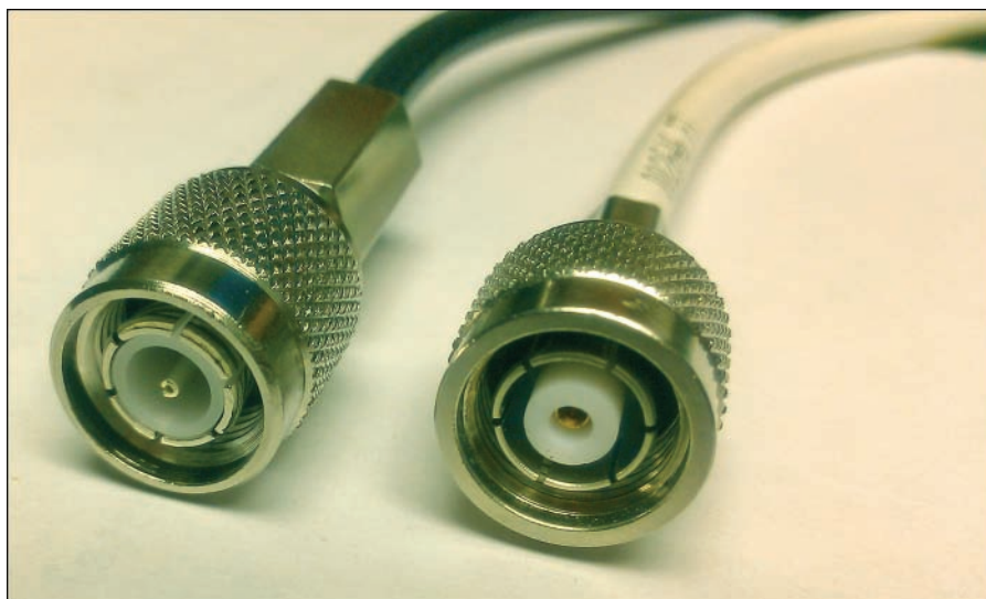
Figure 2-1 Comparison Between TNC (left) and Cisco RP-TNC Connector (right)
