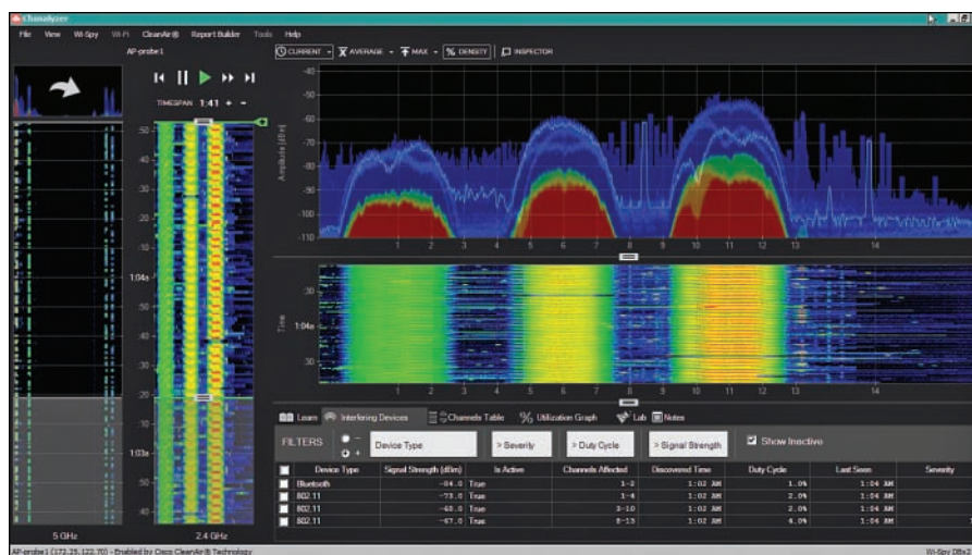
Figure 19-1 Spectrum Analysis with MetaGeek Chanalyzer and a Cisco AP
